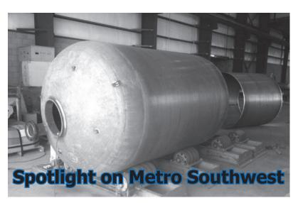
As part of the District's proactive infrastructure maintenance strategy, two old pressure tanks in Metro Southwest are planned for replacement this year. The photo shows the ongoing fabrication process for the new replacement tanks that will enhance reliable service. •
